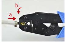
5. a. Put the plug into the crimp tool in the right position.
