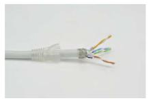
Bend back the copper braid or drain wire over plastic jacket and cut each pair's aluminum foil. (in case of pair shielded cable)
