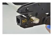
7. Use the crimping tool to clamp the strain relief with cable.
