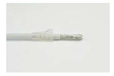
1. Let cable through the boot then strip the cable jacket length about 30mm.
