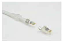
3. Insert the separator and cut the wires straightly and leave the length approximately 15mm.
