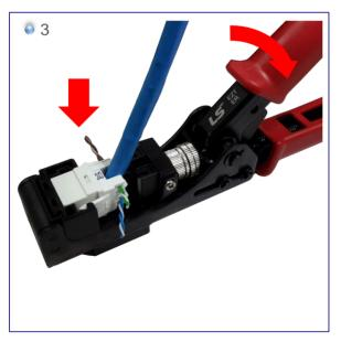
3. Put the Keystone Jack onto the Easy Tool in the right position and then squeeze the tool then terminate all wires and trim the excess wires at the same time.
