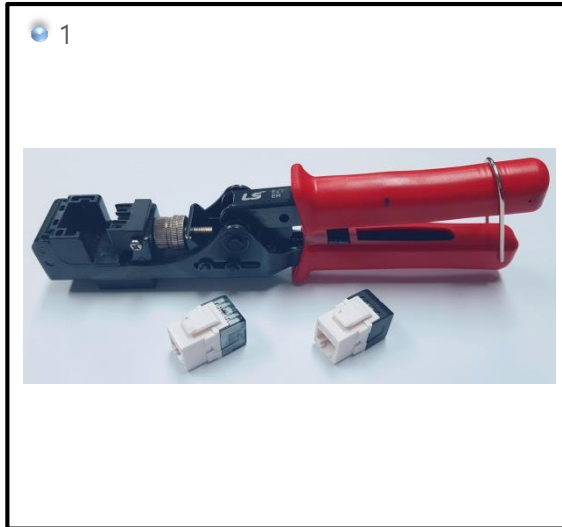
1. Prepare the Easy termination tool with ERI modular jack.
