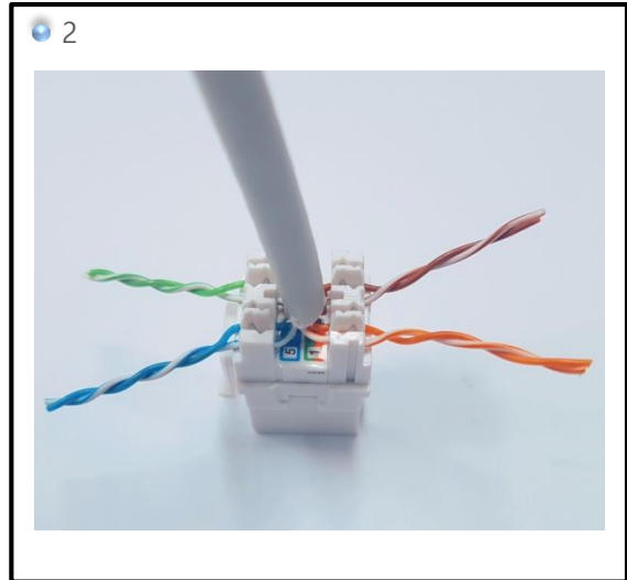
2. Place the wires into the slots according to the wire scheme(T-568A or T-568B)
